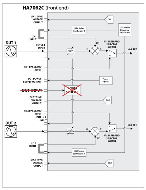
Figure 2: HA7062D Noise Floor Measurement Block Diagram
