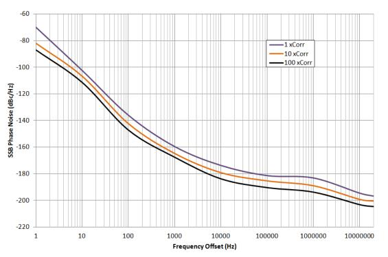
Figure 4: 100MHz Noise Floor Measurements
