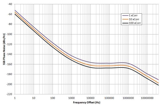
Figure 5: 1GHz Noise Floor Measurements
