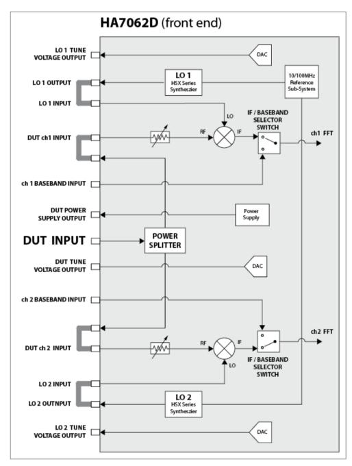
Figure 1: HA7062D Front End Block Diagram
