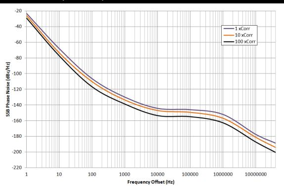
Figure 6: 3GHz Noise Floor Measurements
